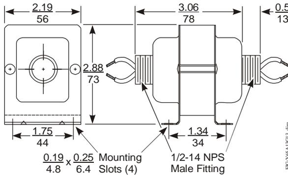
**Figure 2: Dimensions for Y65A13 and Y65G13 Types, in./mm**
