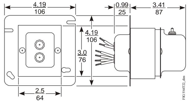
Figure 18: Dimensions for Y64T22 Type, in./mm
