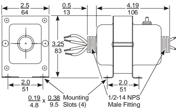
**Figure 13: Dimensions for Y66T13 Type, in./mm**
