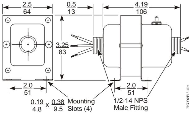
Figure 15: Dimensions for Y66F13 Type, in./mm
