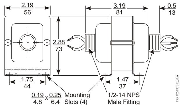
**Figure 7: Dimensions for Y65F13 and Y65S13 Types, in./mm**
