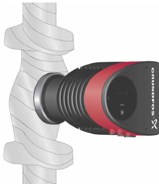
Fig. 13 Insulation of pump housing and pipework
