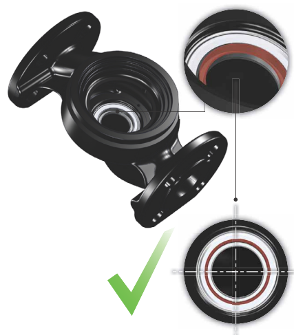
Fig. 10 Correctly centered sealing system
