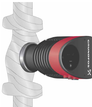
Fig. 13 Insulation of pump housing and pipework
