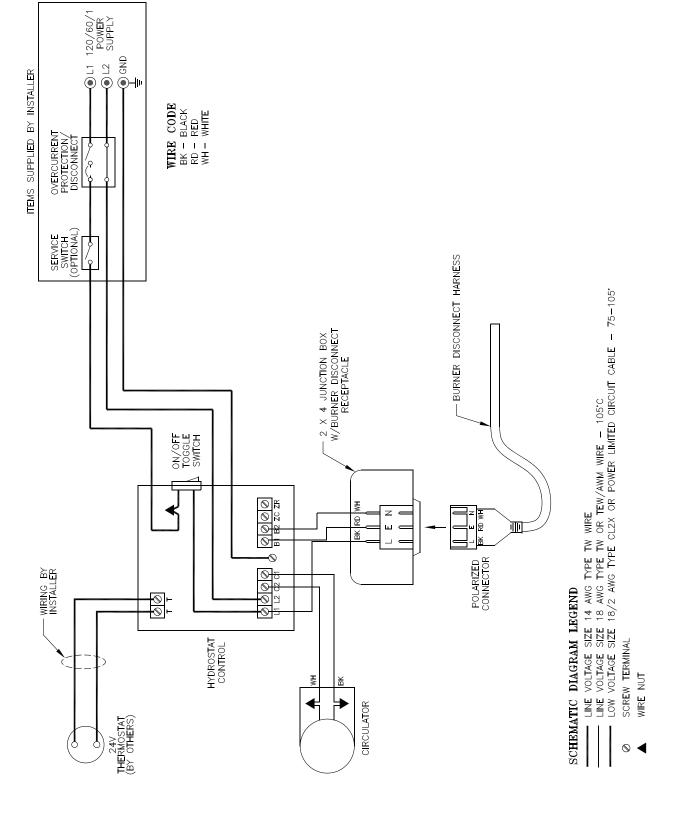
Figure 7-1: Schematic Wiring Diagram, Water Boiler, Hydrolevel Hydrostat (All Burners)
