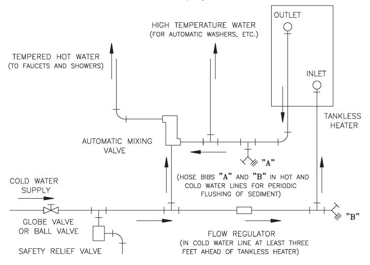
Figure 5-1: Schematic Tankless Heater Piping
