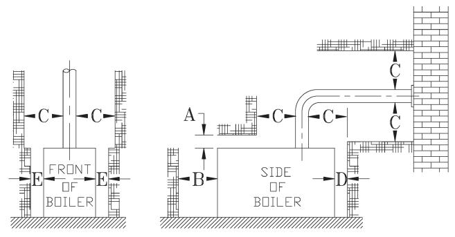
Figure 2-1: Minimum Installation Clearances To Combustible Materials (Inches)
