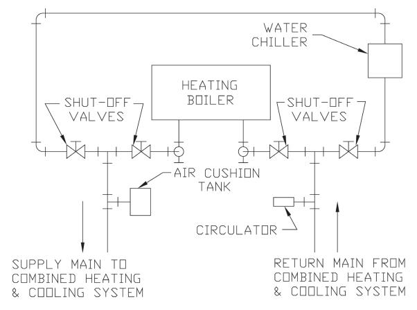
Figure 4-1: Recommended Piping for Combination Heating and Cooling (Refrigeration) System
