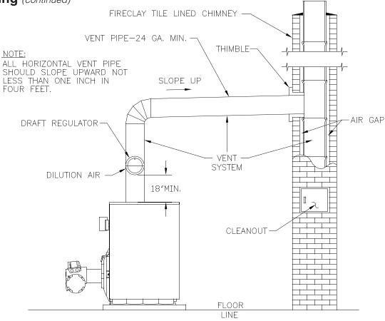
Figure 6-1: Recommended Vent Pipe Arrangement and Chimney Requirements
