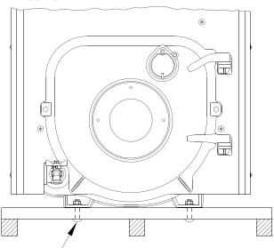
Figure 3-1: Packaged Boiler Removal from Skid
