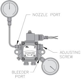
Figure 9-1: Adjusting Fuel Pump Pressure
