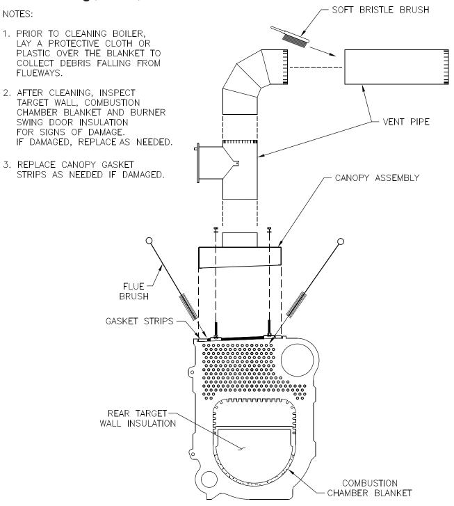
Figure 12-1: Cleaning of Boiler Flueways
