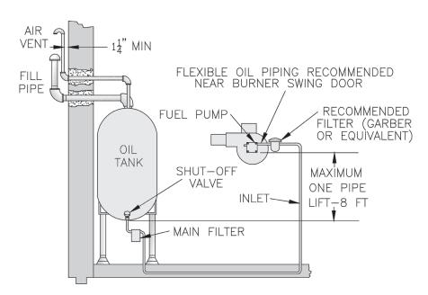
Figure 8-1: Single Pipe Oil Line
