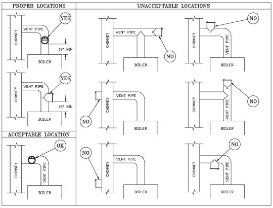
Figure 6-2: Proper and Improper Locations of Draft Regulator
