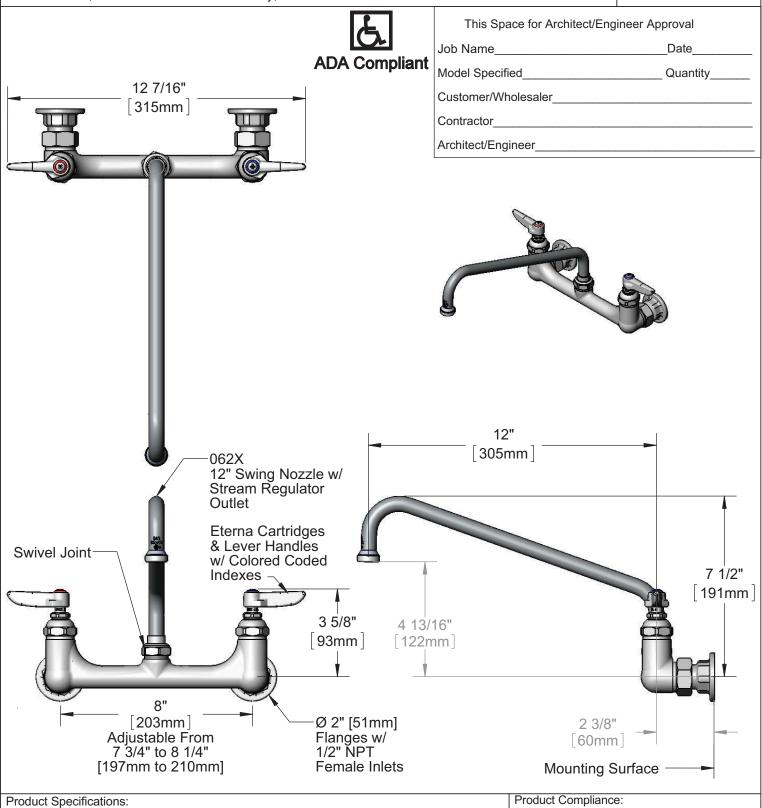
8" Wall Mount Mixing Faucet w/ Eterna Cartridges, Lever Handles, 12" Swing Nozzle & 1/2" NPT Female Inlets
