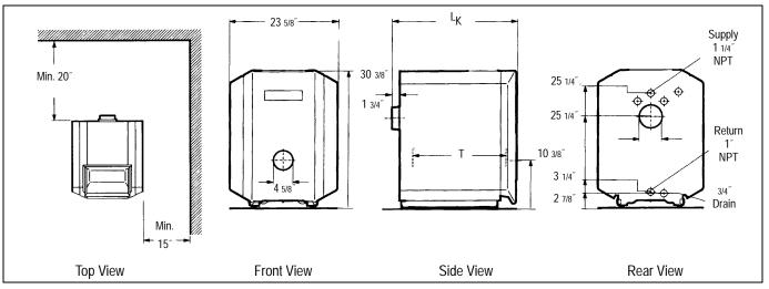
Note: G115 boiler approved for 6" side clearance. Above clearances are recommended for ample access.
