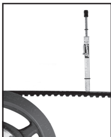
Figure 11: Belt Tension Checker
