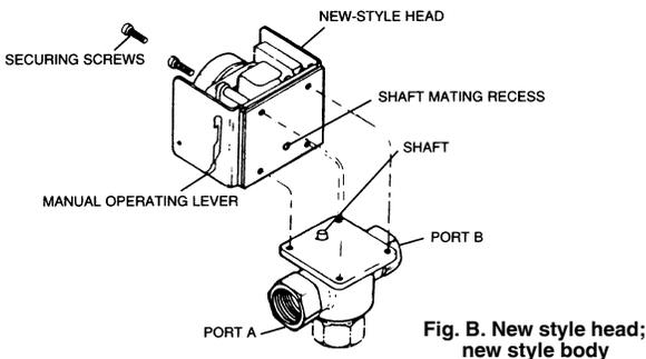
Fig. B. New style head; new style body
