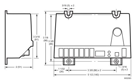
Fig. 2. S8610U module dimensions in inches (mm).
