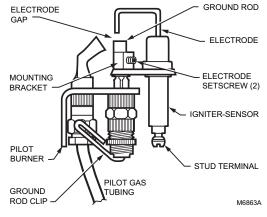
Fig. 9. Fasten igniter-sensor to ground rod.
