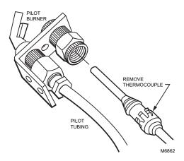
Fig. 7. Remove thermocouple from pilot burner.
