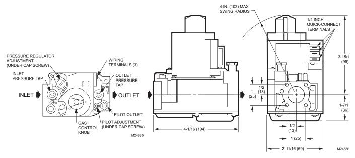
Fig. 3. VR8304M mounting dimensions in inches (mm).
