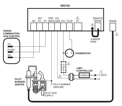
A POWER SUPPLY. PROVIDE DISCONNECT MEANS AND OVERLOAD PROTECTION AS REQUIRED.
