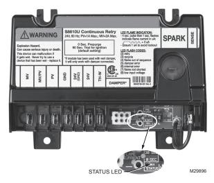
Fig. 21. Location of LEDs.
