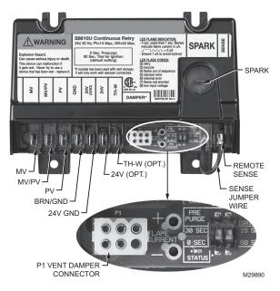
Fig. 15. S8610U Typical wiring connections.
