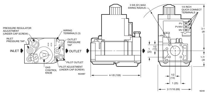
Fig. 4. VR8204A mounting dimensions in inches (mm).
