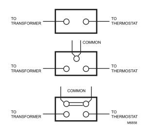
Fig. 6. Wiring connections on standing pilot gas controls.
