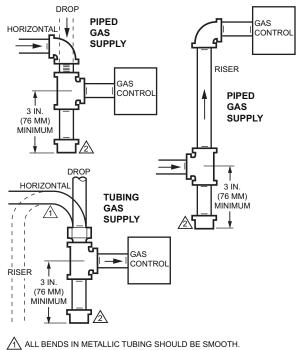
CAUTION: SHUT OFF THE MAIN GAS SUPPLY BEFORE REMOVING END CAP TO PREVENT GAS FROM FILLING THE WORK AREA. TEST FOR GAS LEAKAGE WHEN INSTALLATION IS COMPLETE. M3077A
