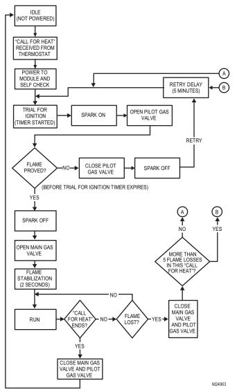
Fig. 19. Normal operating sequence without vent damper.
