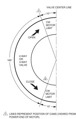
SPRING RETURN MODELS: SPRING DRIVES MOTOR AND VALVE CLOSED IF POWER IS TURNED OFF. M5400
