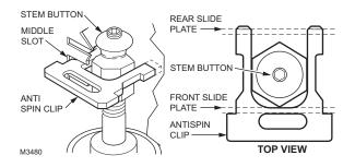
Fig. 2. Installing anti-spin clip
