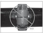
**5.** Visually inspect the bolt pads at each joint to ensure metal-to-metal contact is achieved.
