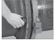
8. JOIN VIC-FLANGE ADAPTER AND MATING FLANGE: Direct the standard, full-shank-diameter assembly bolts, installed in step 7, into the mating flange holes. Hand-tighten a nut onto each bolt to prevent the bolts from pulling out.
