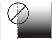
2. The front edge of the pipe end shall be uniform with no concave/convex surface features that will cause improper grooving roll tracking and result in difficulties during coupling assembly (refer to drawing above).
