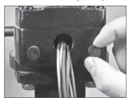
**2.** Remove the travel stop dust cap from the right side of the gear operator, as shown above.
