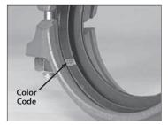
3. CHECK GASKET: Check the gasket to make sure it is suitable for the intended service. The color code identifies the gasket grade. Refer to the "Gasket Selection" section of this manual for the color code chart.
