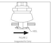
**5. POSITION OUTLET:** Shift the outlet to position the "heel" inside the pipe, as shown in Figure 2 above. **NOTE:** The heel must be positioned, as shown in Figure 2 above, to ensure proper performance under operating conditions.
