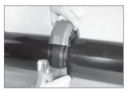
2. **INSTALL HOUSINGS:** Install one side of the hinged housing over the gasket, making sure the keys engage the grooves. Swing the other side of the housing into position. Squeeze the housing to further center the gasket and seat the housing.
