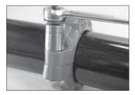
**4. TIGHTEN NUTS:** Tighten the nuts evenly by alternating sides until metal-to-metal contact occurs at the bolt pads. Make sure the housings' keys engage the grooves completely. **NOTE:** It is important to tighten the nuts evenly to prevent gasket pinching.
