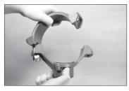
1. ASSEMBLE HOUSINGS: Insert a bolt into the two housings. Thread a nut loosely onto the end of the bolt.
