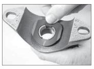
1. INSTALL GASKET: Install the gasket into the gasket pocket, as shown above. Press the gasket along the full circumference to ensure that it seats fully in the gasket pocket. DO NOT LUBRICATE THE GASKET.
