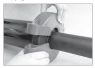
5. INSTALL HOUSINGS: Install the housings over the gasket. Make sure the larger openings of the housings face the larger pipe and that the housings' keys engage the grooves completely on both pipe ends.
