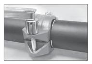
8. TIGHTEN NUTS: Tighten all nuts evenly by alternating sides until the required torque value is achieved at each nut. Refer to the "Style 99 Torque Requirements" table below for the required torque value. The use of a torque wrench is strongly recommended for proper assembly of Style 99 Roust-A-Bout Couplings. NOTE: It is important to tighten all nuts evenly to prevent gasket pinching and to produce bolt pad gaps that are equal on both sides of the coupling.
