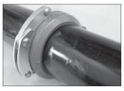
**3a.** Push the locking handle down firmly until the entire handle assembly contacts the coupling housing. The entire handle assembly must contact the coupling housing to ensure a properly locked joint.
