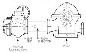
Series 377 Vic-Plug Balancing Valves must be installed with the seat upstream (closest to the pump discharge)
