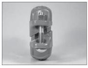
1. DO NOT DISASSEMBLE THE COUPLING: Style 107H Couplings are installation ready. The coupling is designed so that the installer does not need to remove the bolts and nuts for installation. This design facilitates installation by allowing the installer to directly install the grooved end of pipe/mating components into the coupling.
