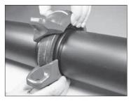
7. INSTALL HOUSINGS: Install the housings over the gasket. Make sure the housings' keys engage the grooves properly on both pipes/mating components.
