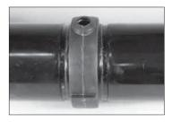
**4. JOIN PIPE ENDS:** Align and bring the two pipe ends together. Slide the gasket into position and center it between the groove in each pipe end. Make sure no portion of the gasket extends into the groove in either pipe end.
