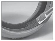
4. LUBRICATE GASKET: Apply a thin coat of Victaulic Lubricant or silicone lubricant only to the sealing lips of the gasket interior. NOTE: The gasket exterior is supplied with a factory-applied lubricant, so there is no need to remove the gasket from the housings to apply additional lubricant to the exterior surface.
