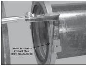
6. TIGHTEN DRAW BOLTS: Torque the draw bolts to approximately 150 ft-lbs/203 N•m to achieve metal-to-metal contact
