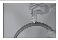
2. CHECK GASKET: Check the gasket to make sure it is suitable for the intended service. The color code identifies the gasket grade. Apply a thin coat of Victaulic lubricant or silicone lubricant to the gasket lips, gasket exterior, and the interior surface of both coupling housings.
