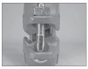
1. DO NOT DISASSEMBLE THE COUPLING: Style 177 Couplings are installation ready. The coupling is designed so that the installer does not need to remove the bolts and nuts for installation. This design facilitates installation by allowing the installer to directly install the grooved end of pipe/mating components into the coupling.
