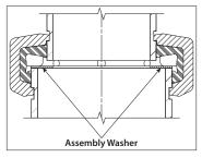
FOR VERTICAL INSTALLATIONS: An assembly washer is recommended to prevent smaller pipe from telescoping inside larger pipe in vertical installations (refer to graphic above). Contact Victaulic for details.
