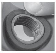
1. CHECK GASKET: Make sure the gasket is seated fully in the gasket pocket. DO NOT LUBRICATE THE GASKET.
