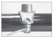
5. TIGHTEN NUTS: Tighten the flange nuts evenly by alternating sides to an approximate torque value of 20 ft-lbs/ 27 N•m to ensure proper gasket compression. NOTE: To avoid overtightening the flange nuts, use a wrench with a maximum length of 8 inches/ 200 mm. DO NOT over-tighten the flange nuts.
