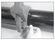
5. INSERT LOCKING PIN: Make sure the proper size locking pin is available (refer to table on this page). Set the locking pin by inserting the plain end of the pin into the hole.
