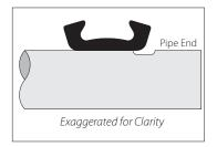
3a. For larger size (non-AGS) couplings (14-inch/355.6-mm and larger): It may be easier to turn the gasket inside out, then slide it over the pipe end. Make sure the gasket does not overhang the pipe end.
