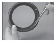
3. LUBRICATE GASKET: Apply a thin coat of Victaulic Lubricant or silicone lubricant to the gasket sealing lips and exterior. It is normal for the gasket surface to have a hazy white appearance after it has been in service.
