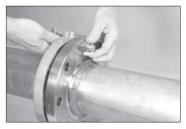
THREAD NUTS ONTO MATING BOLTS: Thread a nut onto each mating bolt. Tighten the nuts until they are fingertight.
