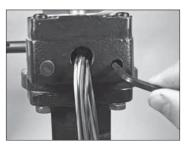
**4.** With the valve disc in the closed (shut) position, tighten the internal set screw (clockwise) with an appropriately sized allen wrench.
