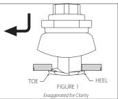
**4. SEAT OUTLET:** Align the "foot" of the outlet with the pipe. Tilt the "toe" into the hole to insert the outlet (refer to Figure 1 above)
