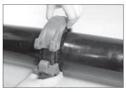
2. INSTALL HOUSINGS: Install one side of the hinged housing over the gasket, making sure the keys engage the grooves. Swing the other side of the housing into position. Squeeze the housings to further center the gasket and seat the housing.
