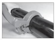
4. ALIGN HOLES: Push the assembly tool down firmly to bring the housings together and to align the holes for the locking pin.
