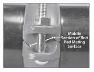
**NOTE:** It is possible to bring the outside sections of the bolt pads into metal-to-metal contact without having metal-to-metal contact at the middle section of the bolt pad mating surfaces. Even tightening of the nuts is required to bring the entire bolt pad sections into metal-to-metal contact. Refer to the graphics on the following page for details.
