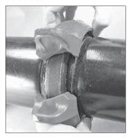
7. INSTALL HOUSINGS: Install the housings over the gasket. Make sure the housings' keys engage the grooves properly on both pipes/mating components.
