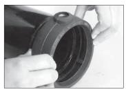
3. INSTALL GASKET: Install the gasket onto the pipe end so that the lips on one side cover the area between the groove and the pipe end. NOTE: The pipe end should not contact the reinforcement ribs inside the gasket.
