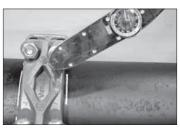
8. TIGHTEN NUTS: Tighten all nuts evenly by alternating sides until the required torque value is achieved at each nut. Refer to the "Style 99 Torque Requirements" table below for the required torque value. The use of a torque wrench is strongly recommended for proper assembly of Style 99 Roust-A-Bout Couplings. NOTE: It is important to tighten all nuts evenly to prevent gasket pinching and to produce bolt pad gaps that are equal at each set of bolt pads.
