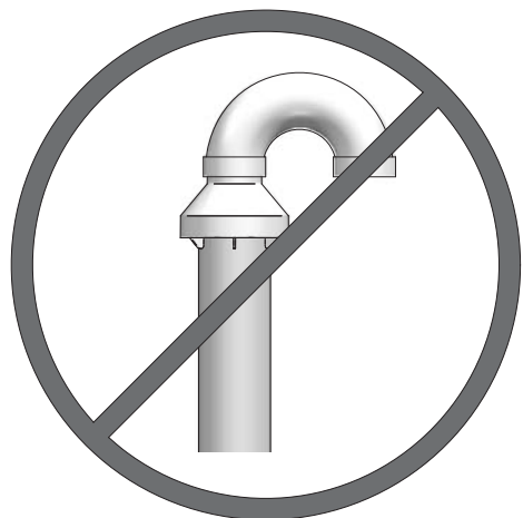
Figure 5-5 Do Not Install U-Bend to Rain Cap
