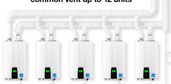
With Navien cascading technology, when a unit gets up to 80% capacity the next unit will turn on to help meet requirements. This demand ratio will continue until all 32 units are generating hot water. The Navien cascading system also balances out the workload of each unit for longer life. Building penetrations are reduced with Navien's common venting feature.
