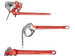
Compound Leverage Wrench – multiplies leverage: used for seized joints
