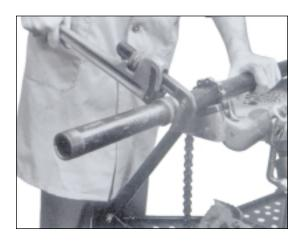
When using a RapidGrip wrench, be sure to center the work piece in the "v" of the hook. If the work piece is not in contact with both sides of the "v", it can reduce wrench gripping action and may result in failure of the hook.
