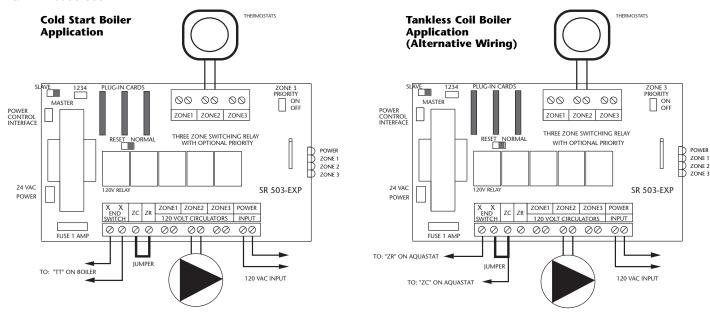
**Warning:** When using Alternative Wiring diagram, wiring instructions must be followed so power originates from the boiler aquastat. Failure to follow these wiring instructions may result in a secondary source of power being connected to the boiler that may activate it under certain circumstances, causing injury or death.
