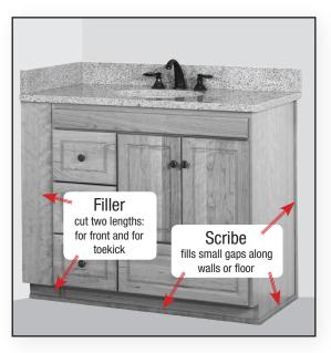
Cut Filler or Scribe to length and secure in place with adhesive or fasteners of your choice.
