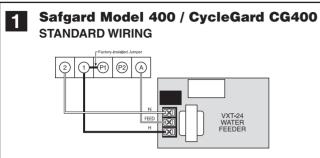
Note: If there is no jumper installed on the low water cut-off between 1 and P1, see ALTERNATE WIRING box.
