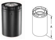
Use to add length to a straight length of DirectVent Pro. 8 ½" pipe adds 3"-7" of length, 16" pipe adds 3"-14 ½" of length, when used with rigid sections of pipe. Direct vent lengths feature a fully unitized, twist-lock construction. Use of sealant is optional, unless specified by the appliance manufacturer. Available in black or galvalume exterior (both feature laser-welded outer wall seams). Does not fit DirectVent GS pipe.
