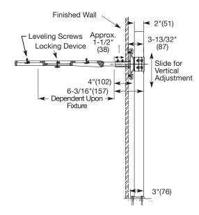
Watts product specifications in U.S. customary units and metric are approximate and are provided for reference only. For precise measurements, please contact Watts Technical Service. Watts reserves the right to change or modify product design, construction, specifications, or materials without prior notice and without incurring any obligation to make such changes and modifications on Watts products previously or subsequently sold.
