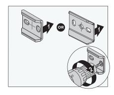
5) Hang top of accessory on mounting bracket. Lower into position.
