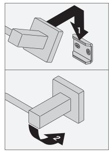
**353-SD2 Only:** Carefully drill 5/16" holes into wall and install anchors. Secure to wall using screws.
