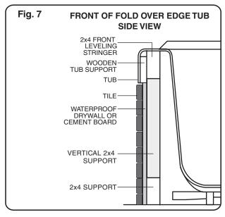
NOTE: Fold Over Tub installations will be butted against the Front Leveling Stringer assembly. See Fig. 7 above (Front of Fold Over Tub - Side View).
