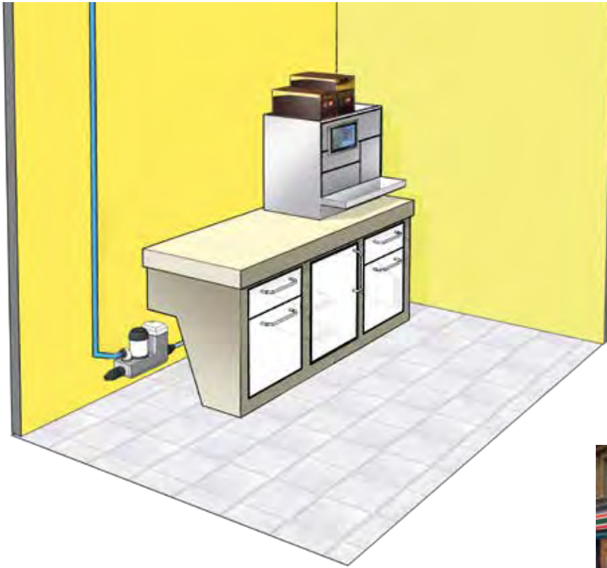
Sanicom installed inside a cabinet with easy access
