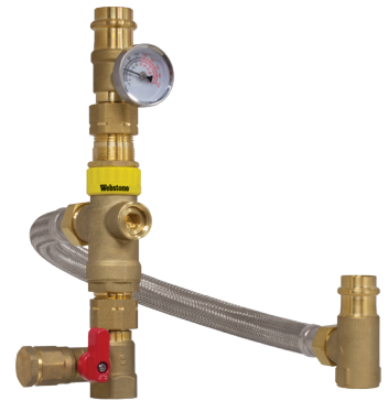
WATER HEATER TEMPERING VALVE W/ TEMPERATURE GAUGE & BY-PASS Forged DZR Brass Valve, w/ 18" Flex Hose Connector, Temperature Gauge, Integral Check Valves & Tempering By-Pass Valve • Outlet Temperature Range 86°-120°F
